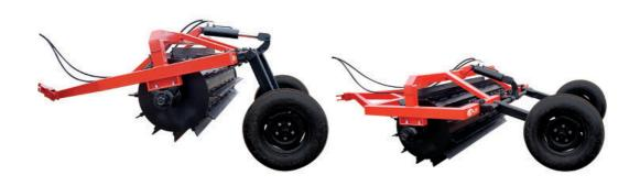
Equipment designed for laid down and / or the incorporation of crop residues; Reinforced Structural chassis with Remote Control; Special Steel Knives with High Resistence; Wheels for transportation hydraulically driven.
